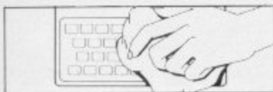
1. Make sure the original keyboard is clean and check that all the keys function.
